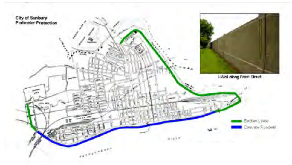
Figure 120: The City of Sunbury, PA, facing repeated flooding from the Susquehanna River, constructed flood walls along its riverfront
